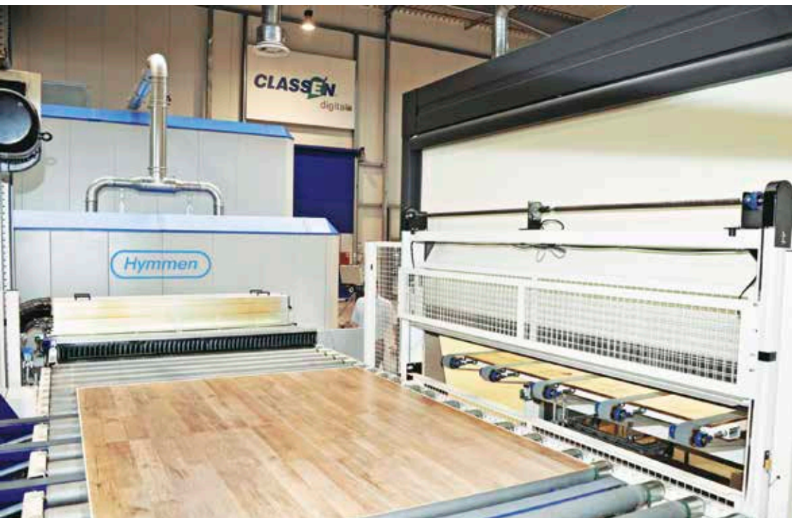
The Hymmen's press digital printing for flooring panel in operation at Classen in Baruth.
